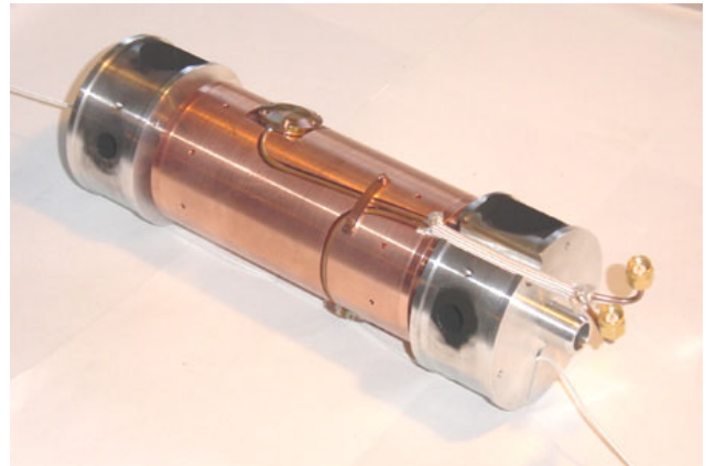
Fig.4 : The resonant cavity and the optical blocks
